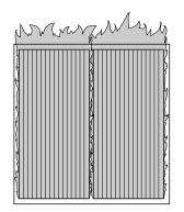
Figure 20 - Incorrect Burner Flame Pattern
